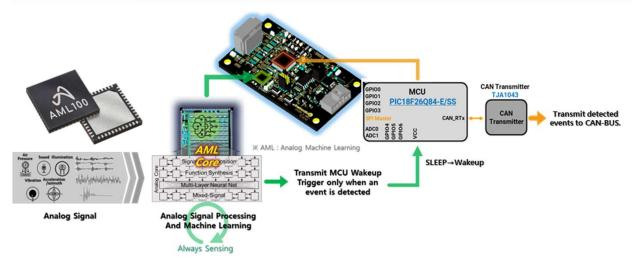
**UAM100** is designed with the Aspinity AML100 chipset of Analog ML process. The Aspinity developed the world fully analog machine learning processor. Also, multiple patents supporting our innovative analog processing/memory.
