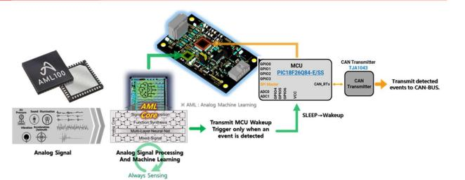
**UAM100** is designed with the Aspinity AML100 chipset of Analog ML process. The Aspinity developed the world fully analog machine learning processor. Also, multiple patents supporting our innovative analog processing/memory.
